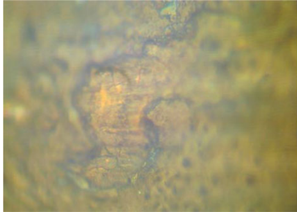
Fig. 20 Epoxy-solid EPDM rubber blend showing a cracked rubber particle
