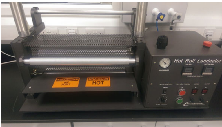
Fig. 5.22 Hot Roll Laminator used to activate PSA
