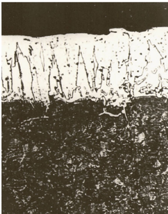
Figure 8.2 The microstructure of the boronized layer in steel 38XC after the liquid non-electrolysis saturation in the bath with boron carbide at 950 °C for 6 h ( \times 200 )
