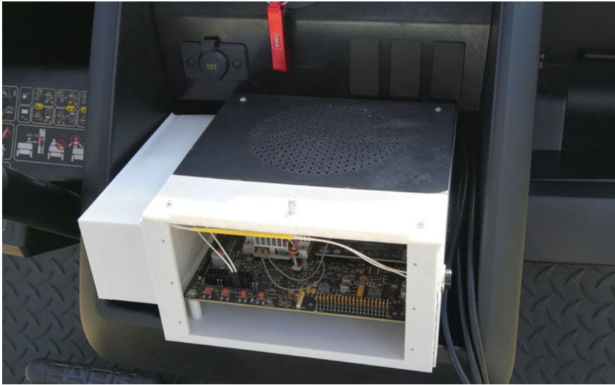
Fig. 3 Jetson TX2 mounted in the front panel of the electric vehicle on a custom 3D printed case. The case also includes a mounting hole for a tripod head to install a camera in case the vehicle used is more compact and space for a battery on the side
