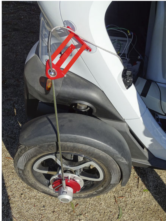
Fig. 12 Installation of an encoder at the rear wheel for positioning purposes
