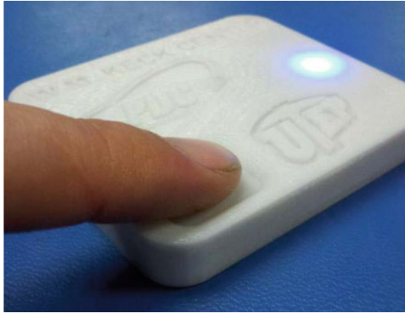
Fig. 7 3D printed capacitive sensors with embedded wire mesh [26]
