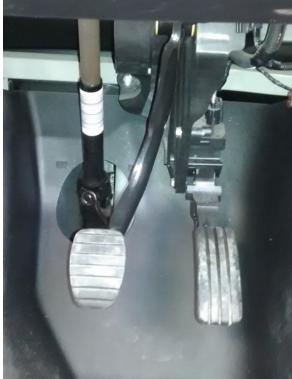
Fig. 8 Original brake and acceleration pedals from the Twizzy
