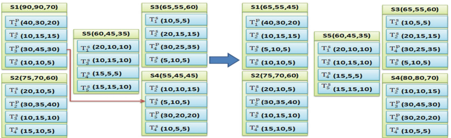
Fig. 4. Load balancing by exchanging the roles between T_3^p at S_1 and T_3^s at S_4
