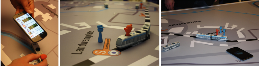
Fig. 2. The interactive Mobia demonstration board including tokens for busses, trams, mobility guides and passengers. The board measures 2.1 m times 1.1 m and is equipped with reed sensors tracking the position of the vehicles.
