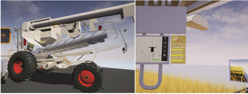
Fig. 4. Examples of prototypes visualizing components of harvesters (left) and UI-concepts for controlling the machine (right).
