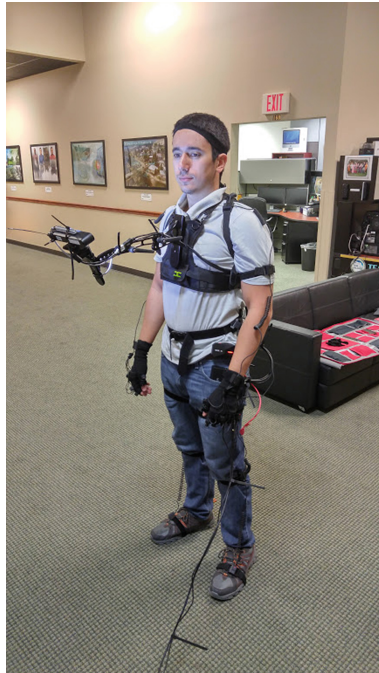
Fig. 2. Wearable markers for full body virtual puppeteering
