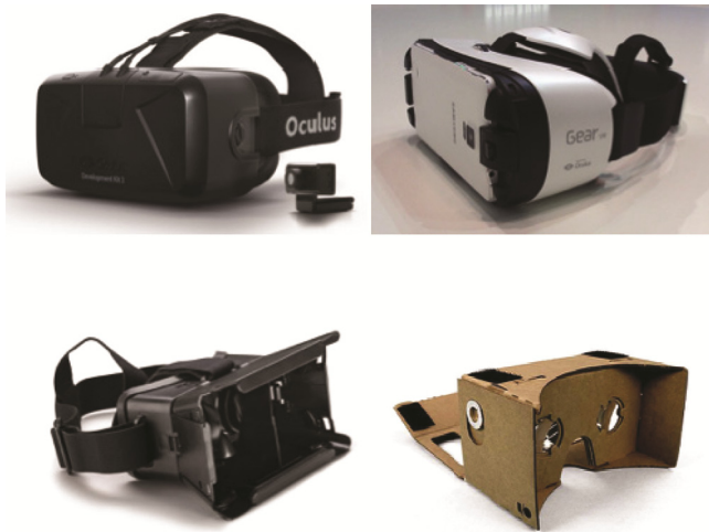
Fig. 1. The Oculus Rift DK2 (top left), Samsung Gear VR (top right), ARCHOS mobile HMD (bottom left), and Do-It-Yourself Cardboard VR (bottom right).
