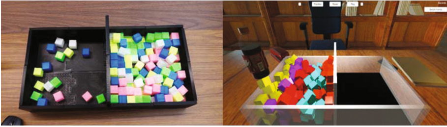
Fig. 1. (Left) Physical version that was 3D printed. (Right) Virtual version that was created in Unity using the Leap Motion.
