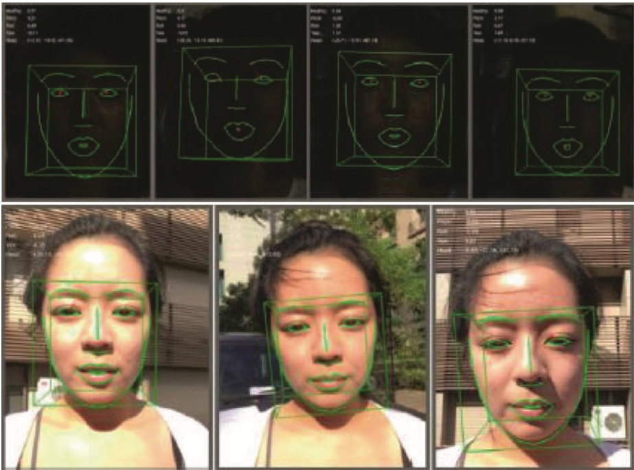
Fig. 8. The facial tracking result under extremely lighting variation (provided by ULSee). Top row: tracking result taken at 0.02 lx. Bottom row: tracking result taken at 46,000-60,000 lx.
