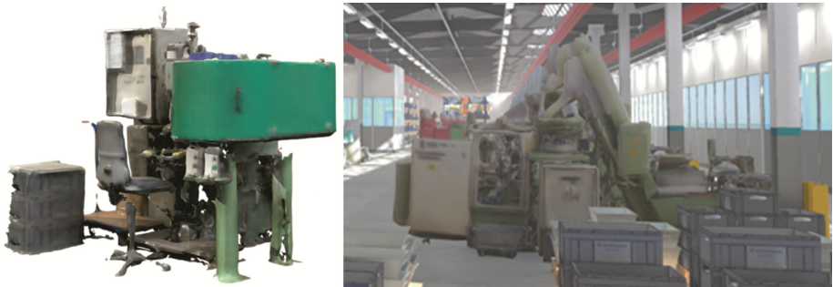
Fig. 3. Scanned 3D model of a production machine (left) and scanned 3D models placed on a factory floor of a production system suitable for an interactive visualization.
