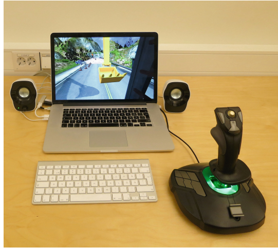
Fig. 4. PC-based simulator, with Bluetooth keyboard and directly connected joystick
