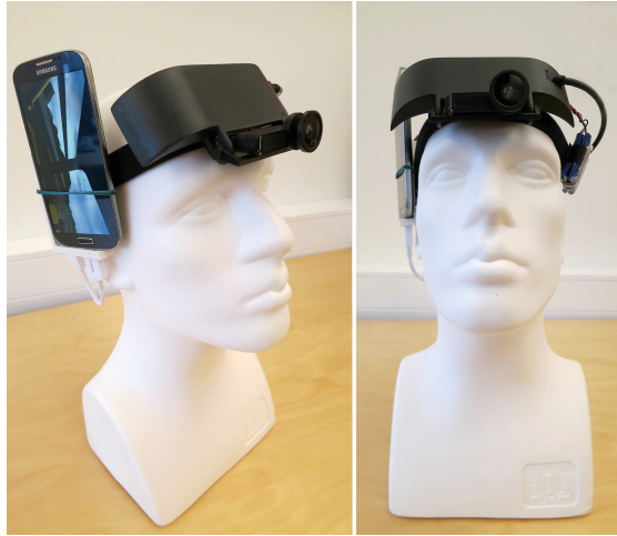
Fig. 1. Picture showing the head-mounted projection display including a smartphone, laser projector with battery pack and 3D printed housing
