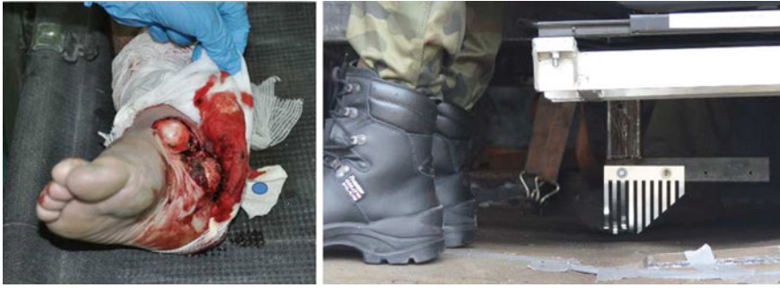
Fig. 1 Left lower leg injury harmed in IED attack on Polish armoured wheeled transporter in Afghanistan [17]; right metal comb—simple device for floor displacement measurement during experiment
