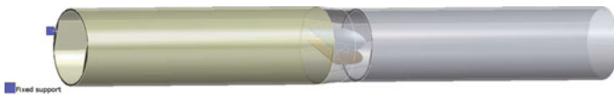
Fig. 6 The fixation of the models presented in the example of the bileaflet heart valve
