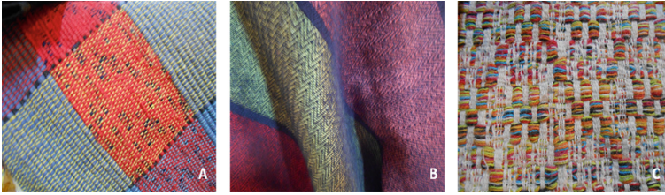
Fig. 5. Handloom – closed thread. The samples (A) and (C) show fabrics of cotton fibre made by a handloom. Sample (B) cloth with acrylic filaments made in a handloom. Source: author's property.
