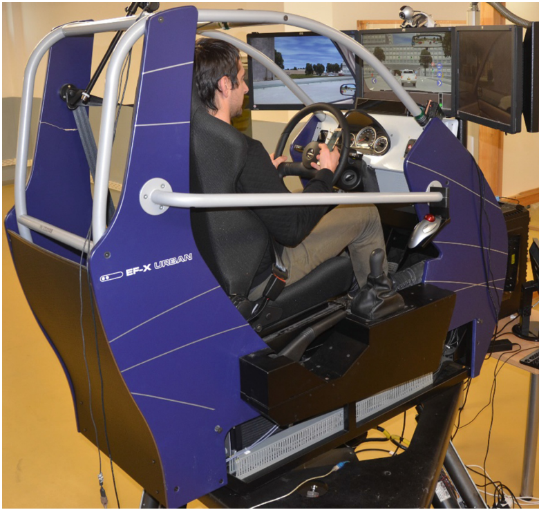
Fig. 3. EF-X Eca-Faros driving simulator
