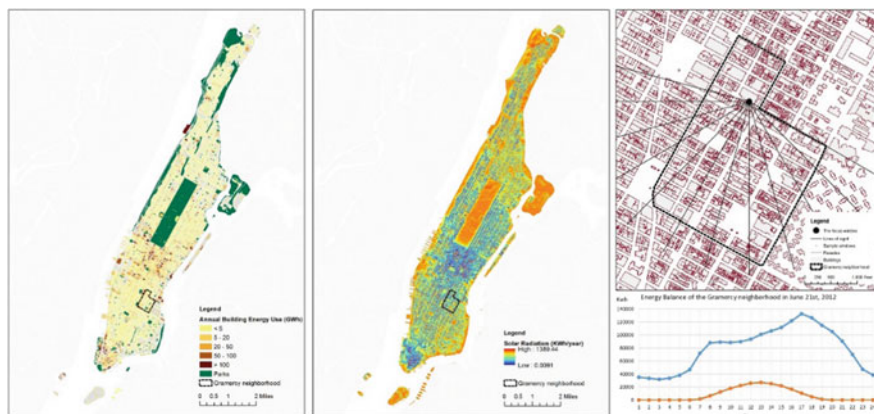
Fig. 9 Urban energy modeling in Manhattan. Left Annual building energy use mapping; Middle Annual solar radiation mapping; Top Right Sample window points on the facades and the lines of sight in Gramercy neighborhood; Bottom Right Aggregated hourly energy balance of solar buildings in Gramercy neighborhood (Quan et al. 2015a)
