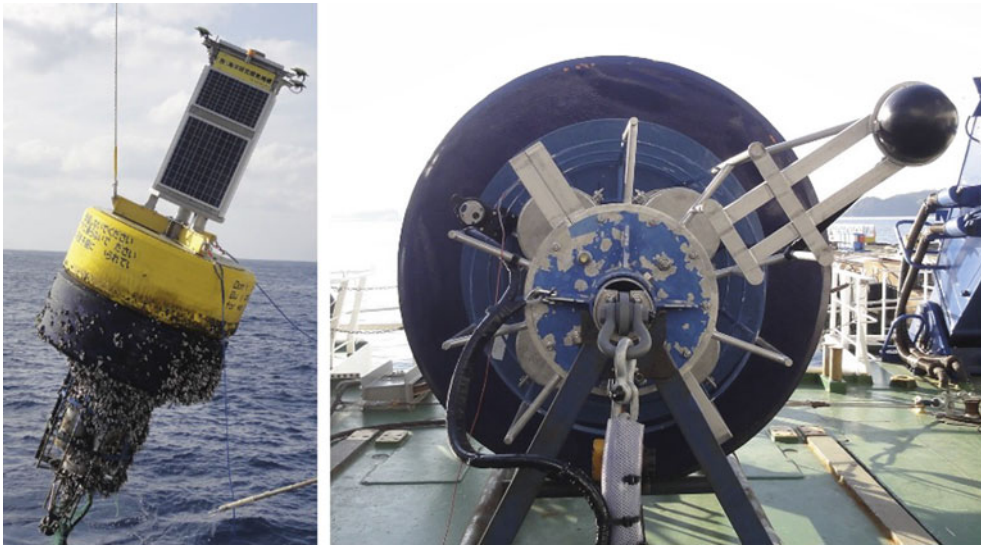
Fig. 4 Whole view of the k-TRITON buoy for the long-term Kumano-nada trials ( left ). An acoustic transducer is equipped at the bottom of the buoy ( right )
