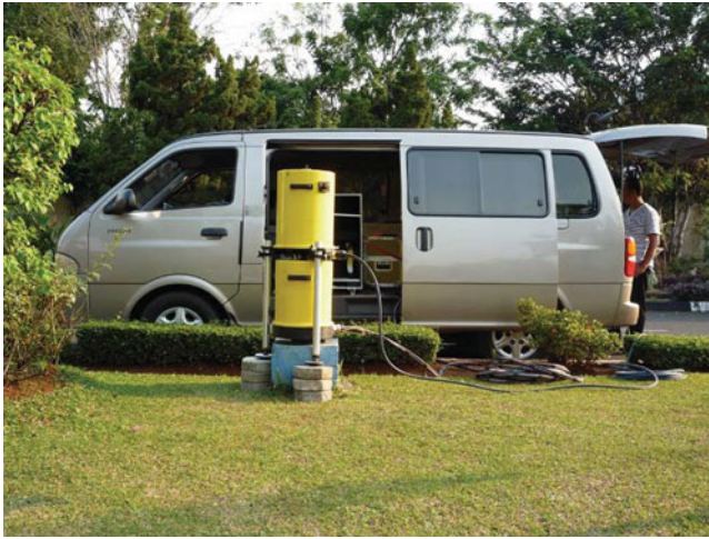
Fig. 1 A photograph of road-side absolute gravity measurements by using A10-017
