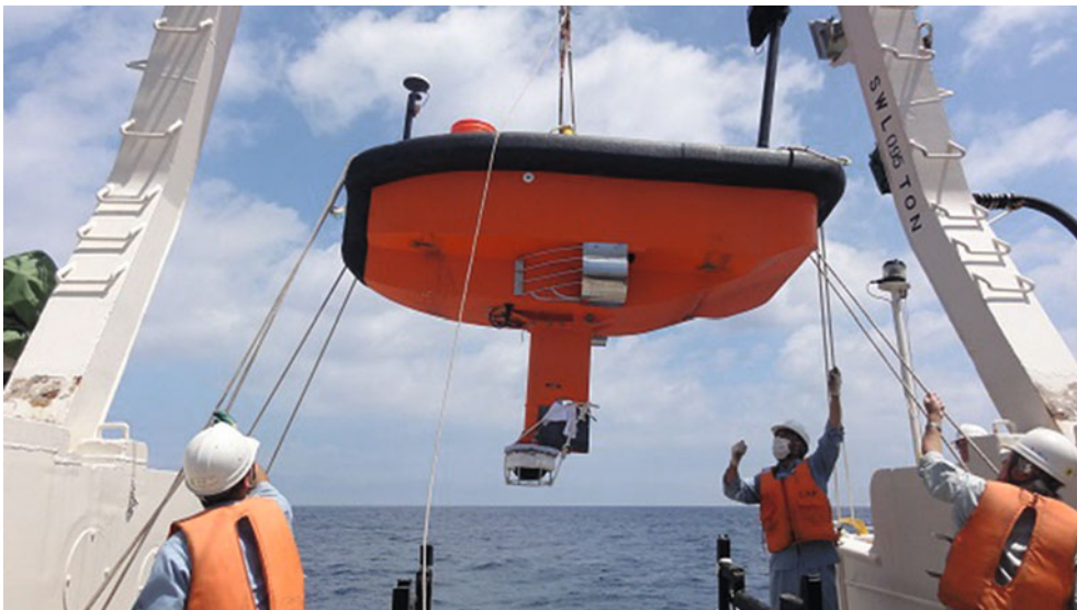
Fig. 5 Deployment of the ASV. The acoustic transducer is at the lower end of the keel
