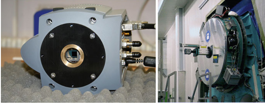
Fig. 1.9 AstraLux Sur: ANDOR iXon+ DU-897 camera ( left ), instrument attached to the adaptor rotator of the ESO 3.5 m NTT ( right ) (Reproduced with permission from [15])
