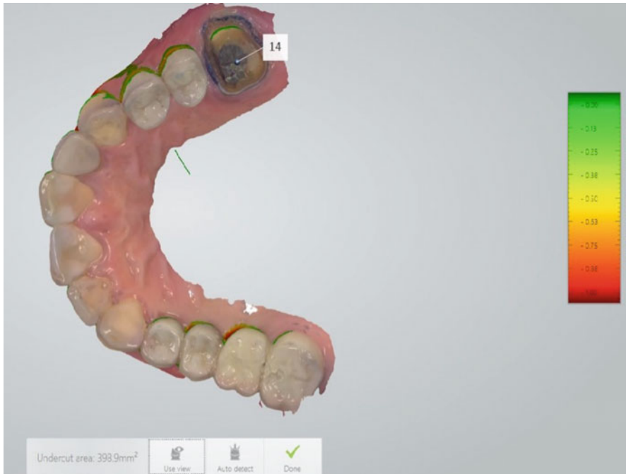
Fig. 11.5 Undercut detection shown in green
