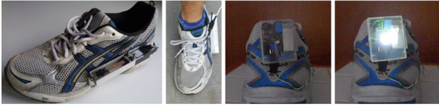
Fig. 16 Piezoelectric device placed in center of the shoe in an aluminum structure, the system with a led has been placed in the back of the shoe
