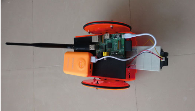
Fig. 2 Embedded robotic platform: differential wheeled robot and Raspberry Pi
