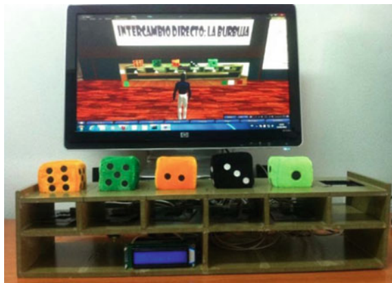
Fig. 1 Virtual Touch toolkit teaching sorting methods using physical dices
