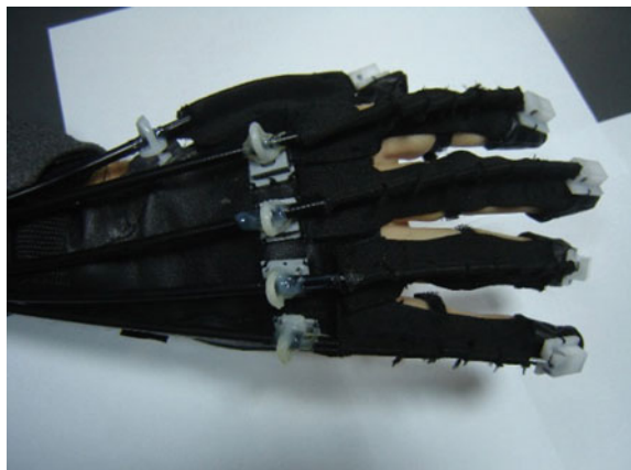
Fig. 4 Wearable soft robotic glove with Bowden tendons
