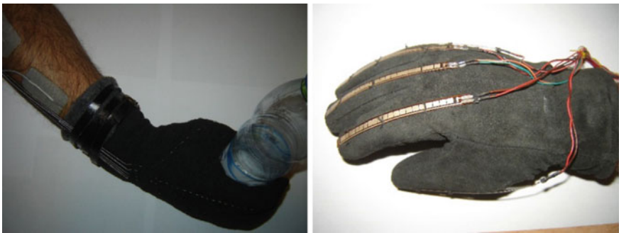
Fig. 7 Robotic glove and FES. Tele-operation glove with flex sensors
