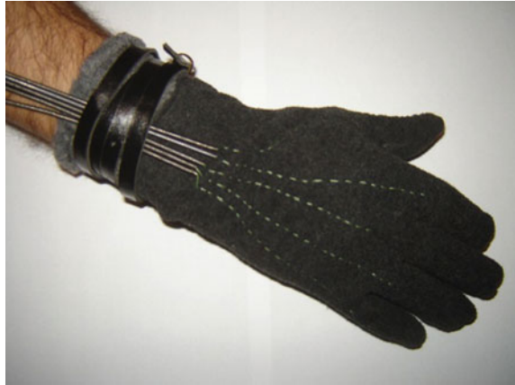
Fig. 5 Wearable soft robotic glove with flexible tendons
