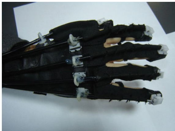
Fig. 4 Wearable soft robotic glove with Bowden tendons
