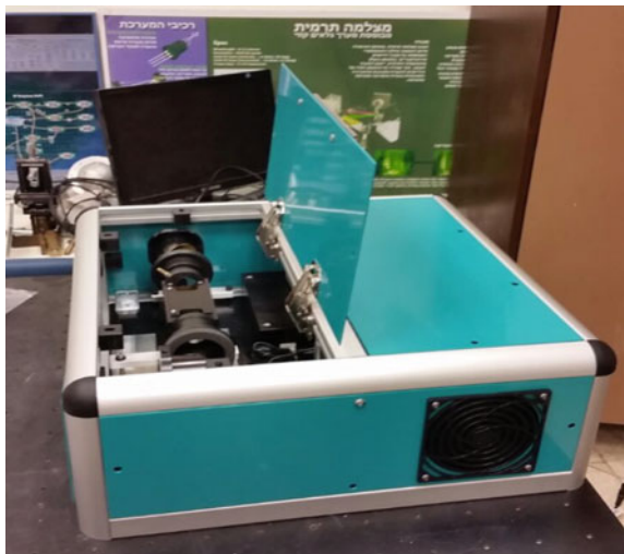
Fig. 3 The open view on an in-vitro operated MIR-ATR system
