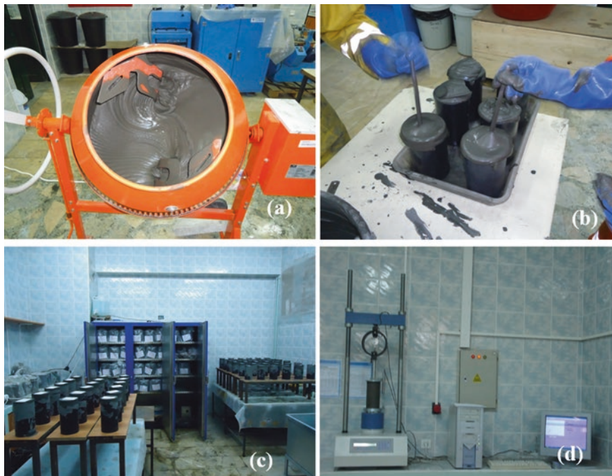
Fig. 2.4 Laboratory-scale tests of paste backfill materials: (a) preparation of the mixture, (b) tamping, (c) curing and (d) uniaxial compressive and deformation testing
