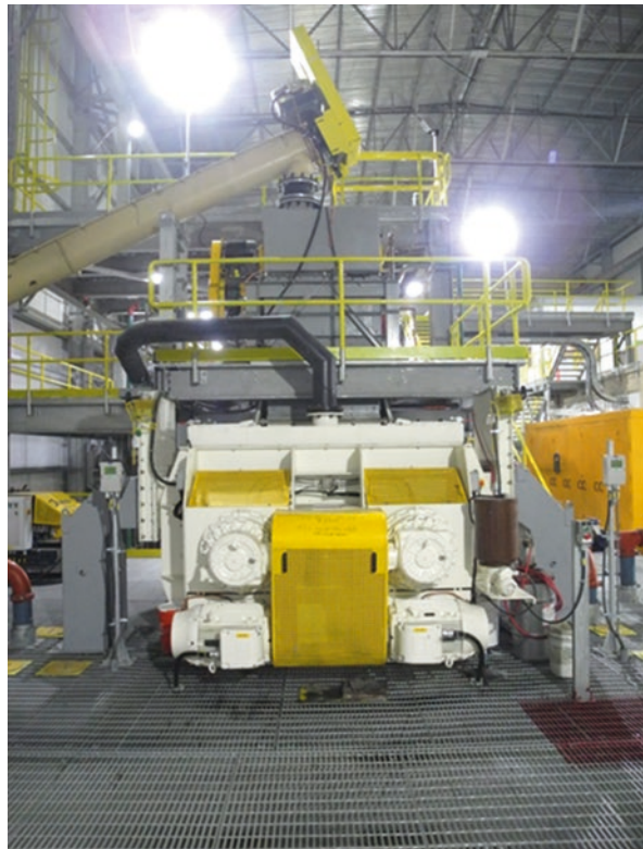
Fig. 12.4 Continuous mixer view from the discharge end illustrating the binder screw conveyor feed, dual-side discharge chutes and planetary drive system of the twin-shaft mixer
