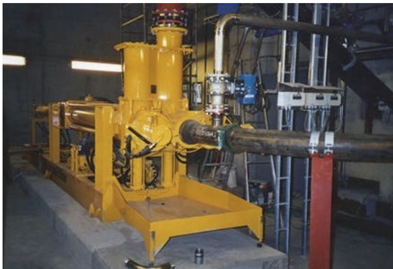
Fig. 5.14 Paste backfill being pumped underground using Putzmeister pump
