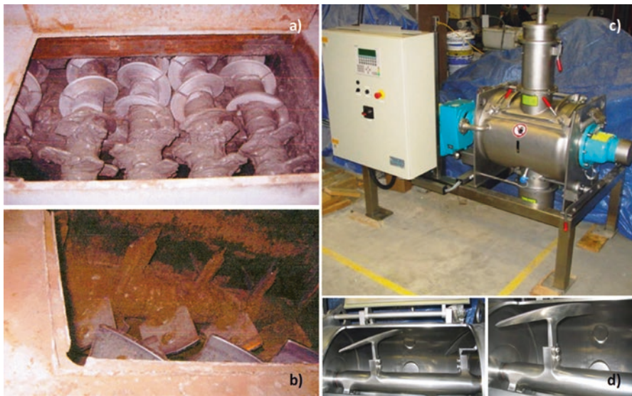
Fig. 5.12 Photos of (a) screw-type, (b) paddle-type, (c) plowshare or plow mixers, and (d) special shovels of plowshare mixer (modified from Dirige et al., 2008.)
