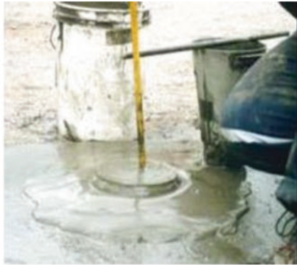
250 mm (10 inch) slump paste tailings
