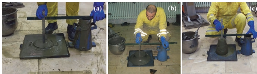
Fig. 2.7 Slump with (a) a high value, (b) a normal value and (c) and a low value
