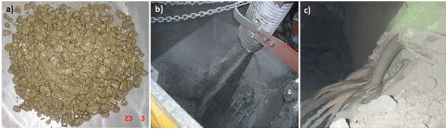
Fig. 5.1 Mine backfill methods: (a) rock, (b) slurry, and (c) paste
