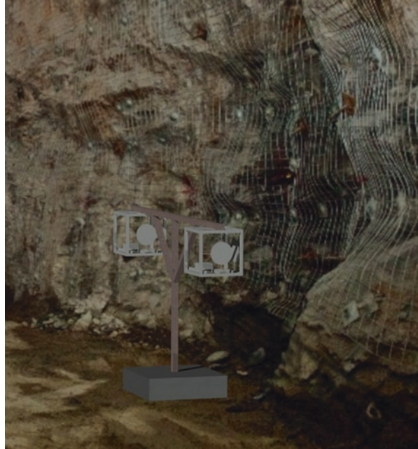
Fig. 7.6 Instrument clusters mounted on T-support structure concept
