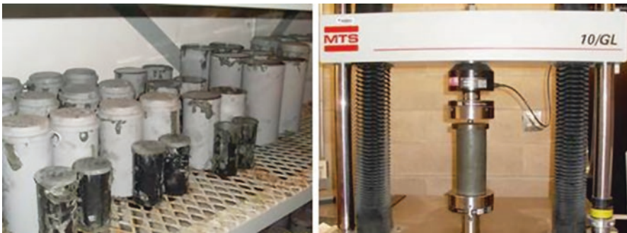
Fig. 5.24 CPB samples cured in a foggy room ( left ) and tested under a UCS test press ( right )
