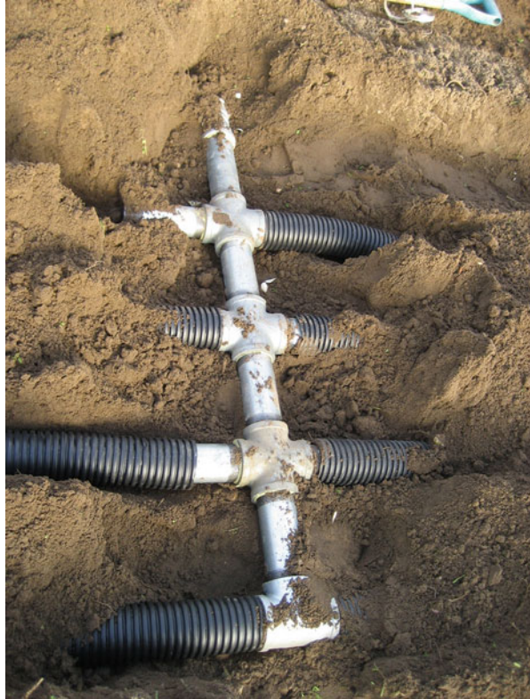
Fig. 14 Steam can be delivered to the field using a fixed boiler system that is attached to buried drain tile. The drain tile is attached to a manifold (seen here) that is connected to the boiler through heat-resistant hose (S. Fennimore © 2017. All Rights Reserved.)
