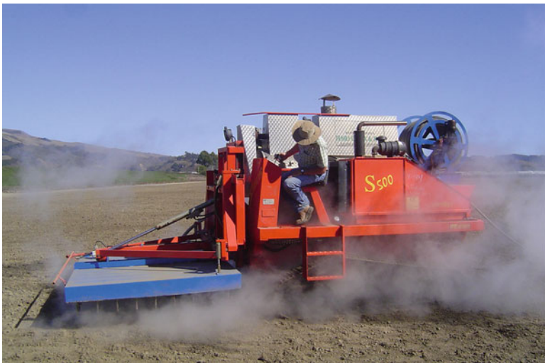
Fig. 16 Numerous commercial mobile steam units are available that mix soil with steam as it moves through the field (S. Fennimore © 2017. All Rights Reserved.)
