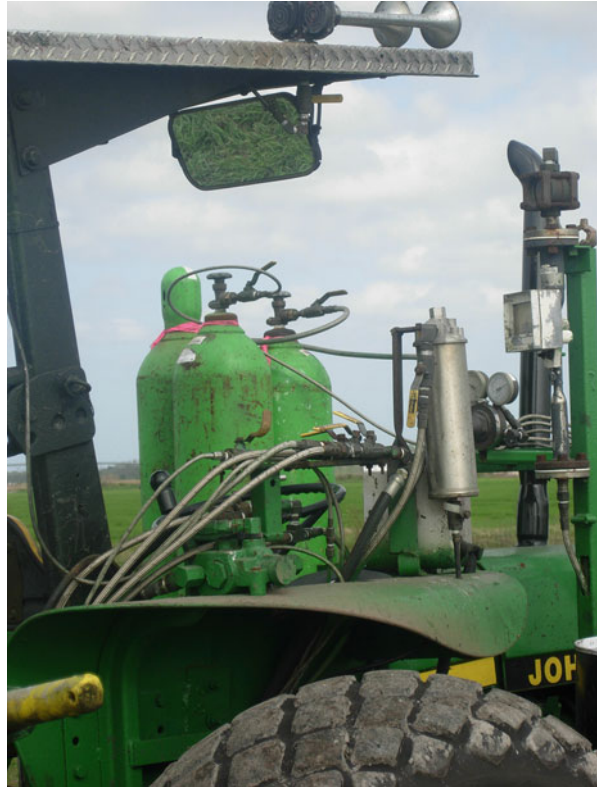
Fig. 9 Fumigants are injected into soil through a series of specialized tubes that are pressurized using nitrogen gas. Different fumigants are delivered with different sizes of tubing and flow meters in order to achieve precise application amounts and effective distribution of material (E. Roskopf. USDA.)
