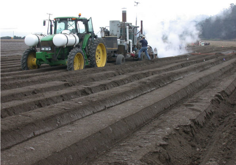
Fig. 17 Large-scale application of steaming requires mobile units with access to water and fuel (S. Fennimore © 2017. All Rights Reserved.)
