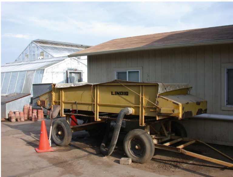
Fig. 5 Soil cart used for steaming potting mix (S. Fennimore © 2017. All Rights Reserved.)
