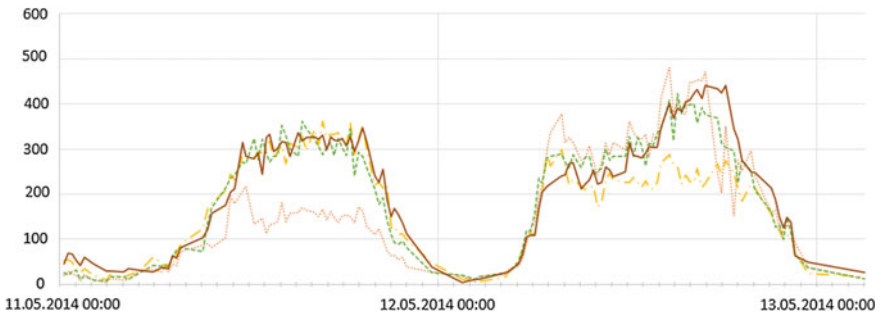
Fig. 6 Input data for the net-traffic flow intensity travel route: Hallera-Lotnicza, first 2 days, each series represents data from one video detection camera, 4 of 8 cameras on the route are presented for clarity
