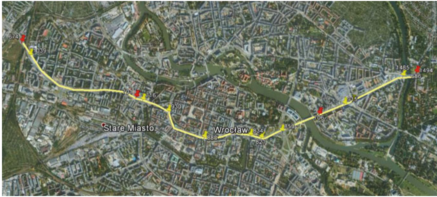
Fig. 4 An example of a travel route (Kochanowskiego–Lotnicza) used for travel time estimation. Red pins ARTR cameras, yellow pins video detection cameras, image: Google Earth
