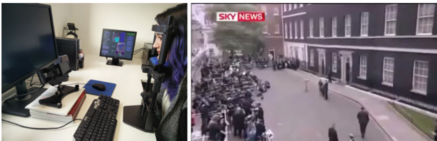
Fig. 1 The experiment recorded participants' eye movements using a remote eye tracker while watching short video clips
