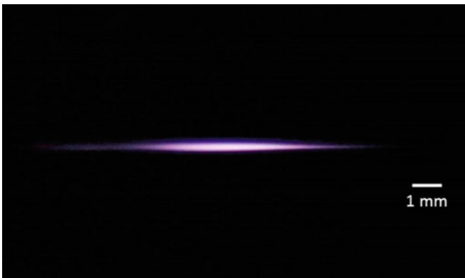
Fig. 6.1 Typical filament formed in water upon its irradiation by a focused beam of 35 fs long pulses of 800 nm light of incident energy 0.3 mJ. The incident laser light was linearly polarized
