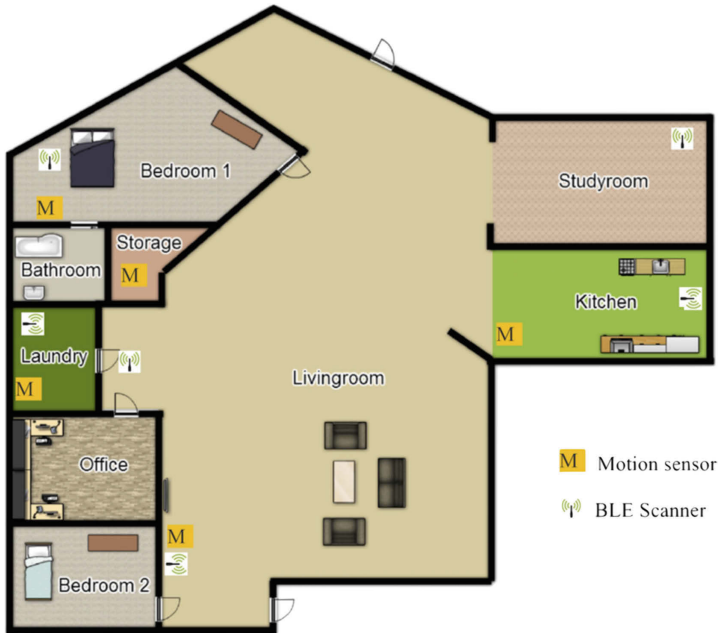
Fig. 2. A dual occupancy smart home with motion sensors and BLE scanners
