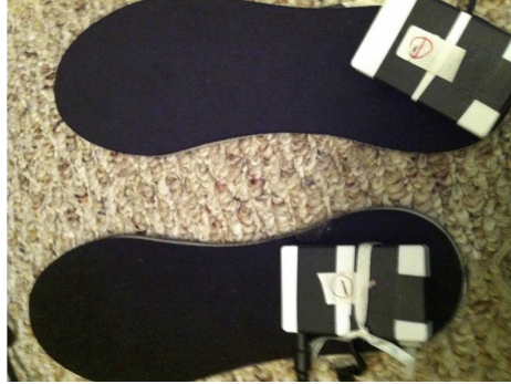
Fig. 2. Sensor system inside the sole of shoes.
