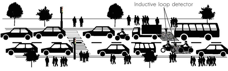
Fig. 1. Inductive loop detector for Traffic Control
