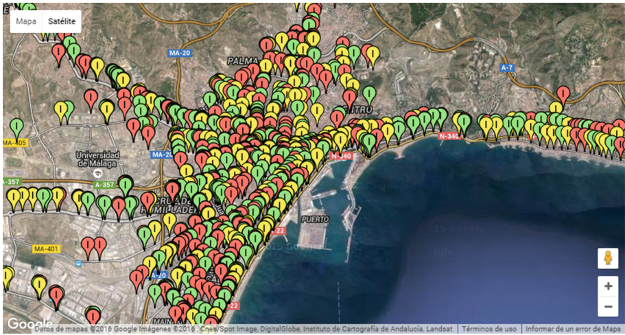
Fig. 3. Differences between base plan and the optimized traffic lights in whole Málaga city map (with 961 intersections). Red color indicates a big difference, yellow a medium one, and green a small one. (Color figure online)
