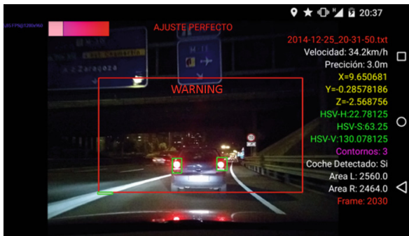
Fig. 2. The application shows information about the velocity, distance, spatial location, HSV colour components, detections and warnings in real time.
