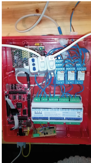
(b) Energy Switch core, internal view
