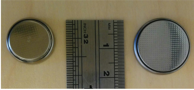
Fig. 4. The two standard coin batteries we used. Left: CR1616 (16 mm diameter, 1.6 mm thickness, \approx 55 mAh). Right: CR2032 (20 mm diameter, 3.2 mm thickness, \approx 230 mAh).
