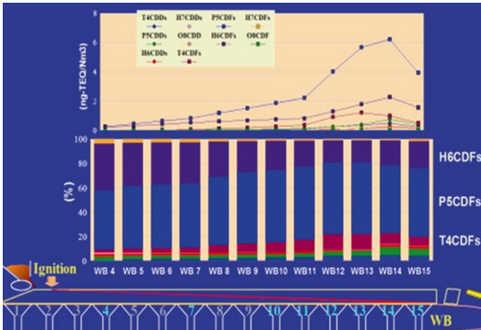
Fig. 5.14 Concentration and fraction of PCDD/PCDFs (TEQ) at the wind boxes of the sinter machine (Kasai, 2002)
