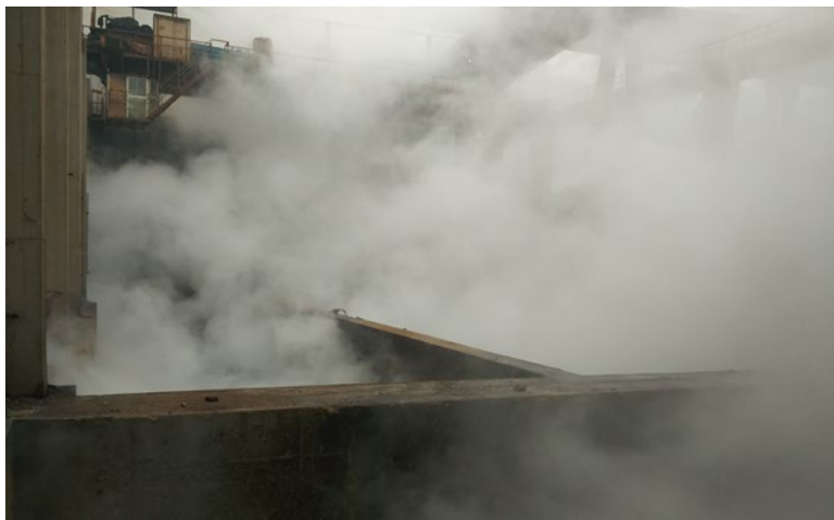
Fig. 7.1 Steam generation in a water granulation process of molten slag
