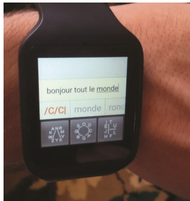
Fig. 2. The UniWatch keypad: text entry approach by button tapping
