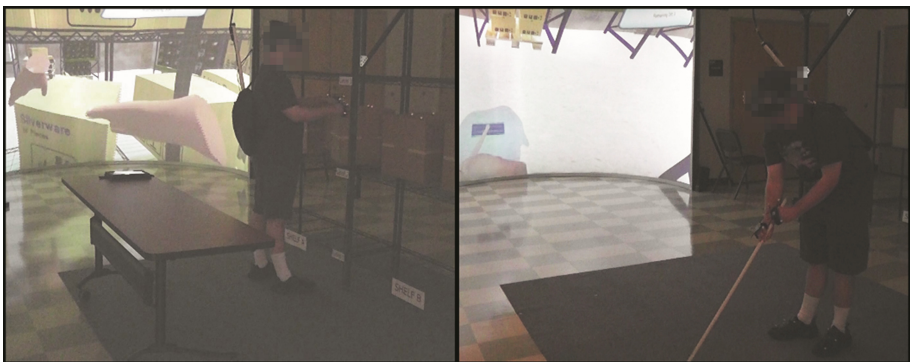
Fig. 1. Tangible object manipulation. Left: the user rotates a real box in shelving tasks. Right: the user uses a broomstick as a virtual mop in cleaning tasks.
