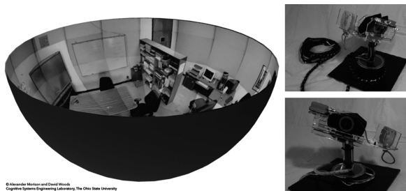
Fig. 4. A panoramic representation created from a narrow field-of-view PTZ camera (left) and two views of a viewpoint control input device or 3-dimensional joystick (right).
