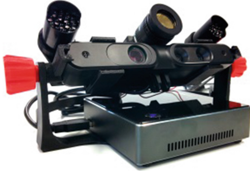
Fig. 1. Eye tracker setup with high resolution Flea3 camera, Asus Xtion, IR Led clusters and processing unit.
