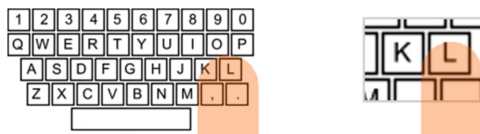
Fig. 4. The ZoomBoard. When the user taps on the miniature QWERTY keyboard, it iteratively magnifies the touched region. The user then can tap on a particular key to enter the corresponding character. The keyboard goes back to its original state immediately after that.
