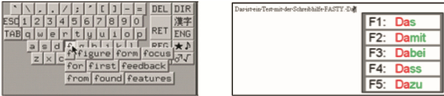
Fig. 1. On the left, PO-BOX interface: when selecting a character, the list appears directly on it. On the right, FASTY interface, the list appears next to the cursor.
