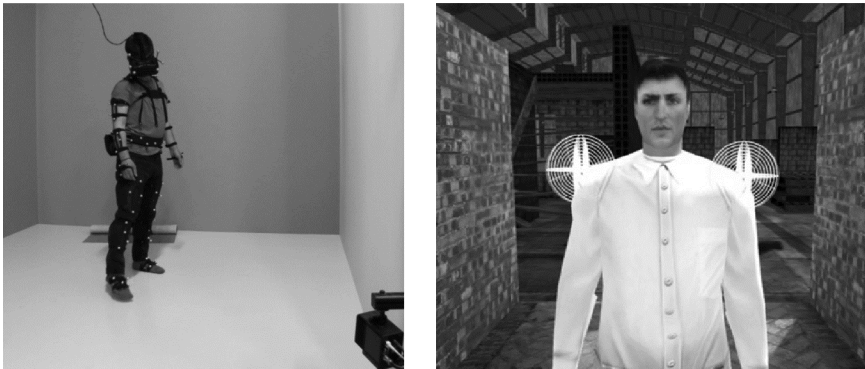
Fig. 1. Left. A subject in the experimental setup. He wears the HMD, equipped with an ART target for the tracking of the head's translational movements. He also wears an ART all-body capture set. Right. The recording of all-body movements are used to build a co-localized avatar (the subject's head was not actually represented in the experiment). The spheres' centers represent the vibrating actuators position on the subject's shoulder. Their size represents the spatial domain in which the actuators were active (that is when the subject shoulder's distance to a virtual object was inferior to their radius). See text for details.
