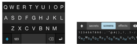
Fig. 7. Screenshots of Fleksy and Minuum, respectively. Both are predictive techniques that correct and disambiguate input at both character and word levels based on the sequence of keys pressed.
