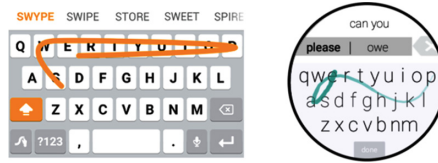
Fig. 8. Screenshots of Swype and WatchWriter [13], respectively. Both are predictive techniques that enable gesture typing. The user enters one character per tap or one word per gesture. The traces in the picture indicate the gestures drawn to enter ‘Swype’ and ‘please’, respectively.
