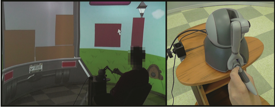
Fig. 2. Haptic device interaction technique. Left: the user holds boxes with the haptic device. Right: the haptic device.
