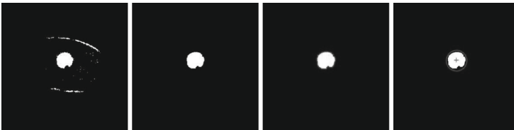
Fig. 5. From left to right: Initial extraction of the pupil, erosion to remove scattered foreground pixels, analysis of blob area, center and minimum enclosing circle
