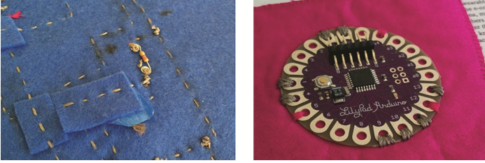
Fig. 3. The system is composed of soft circuits (left) with LilyPad Arduino (right)
