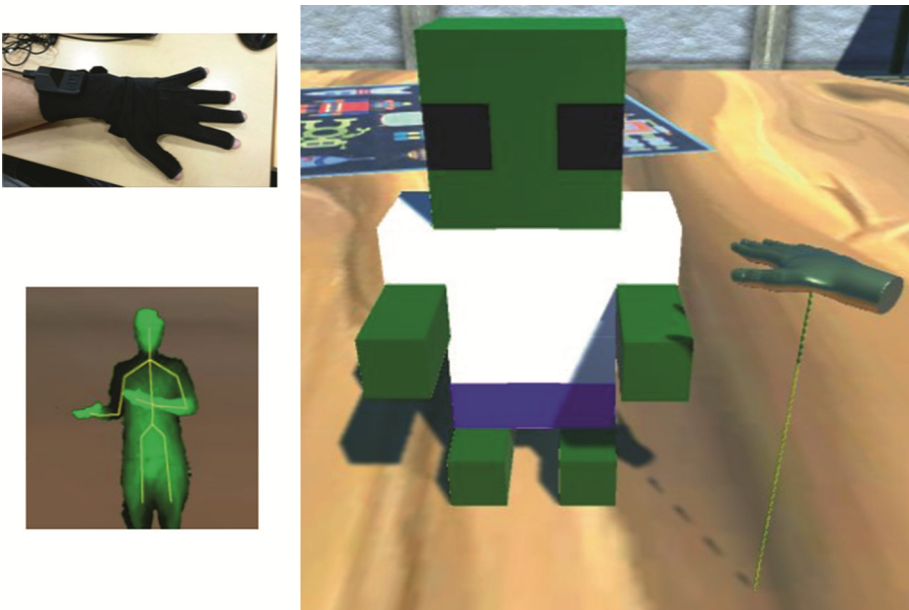
Fig. 5. In the “Créa-Main” project, the virtual hand (right) is controlled by a combination of Kinect and Dat Glove controllers.
