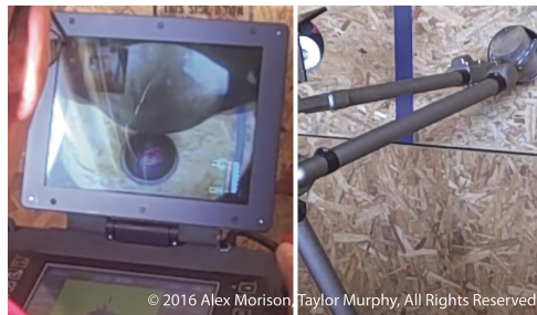
Fig. 1. Operator using a robotic platform with manipulator arm to pick up a cylinder and place it into a similarly sized aperture such that the cylinder would not fall back out in NIST test case. Performance was very poor in general and virtually impossible when the teleoperator could not directly see the robot arm. Note: the two images shown here are of two different robotic platforms.
