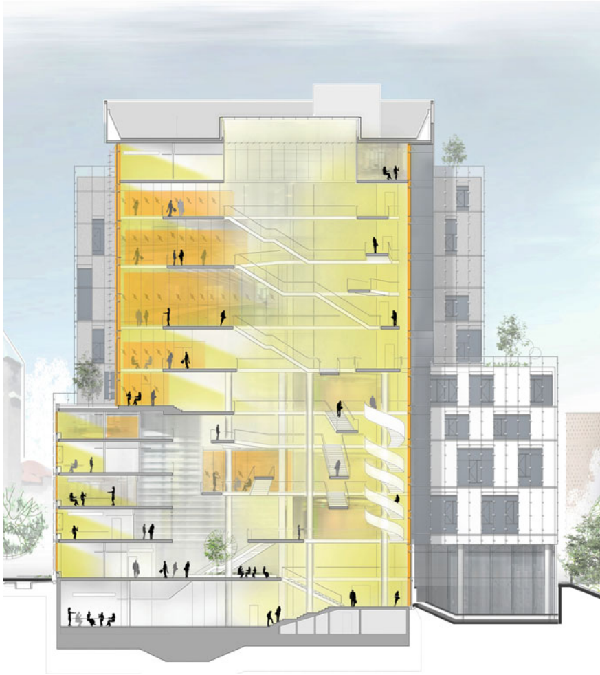
Fig. 1.3 Building section of the John & Frances Angelos Law Center showing the side and top-lit daylight atrium space that serves as the primary means of circulation. Image credit Behnisch Architekten
