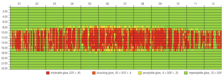
Fig. 2.34 Annual Daylight Glare Probability (DGP) simulation result for window-facing view orientation. Image credit Alstan Jakubiec
