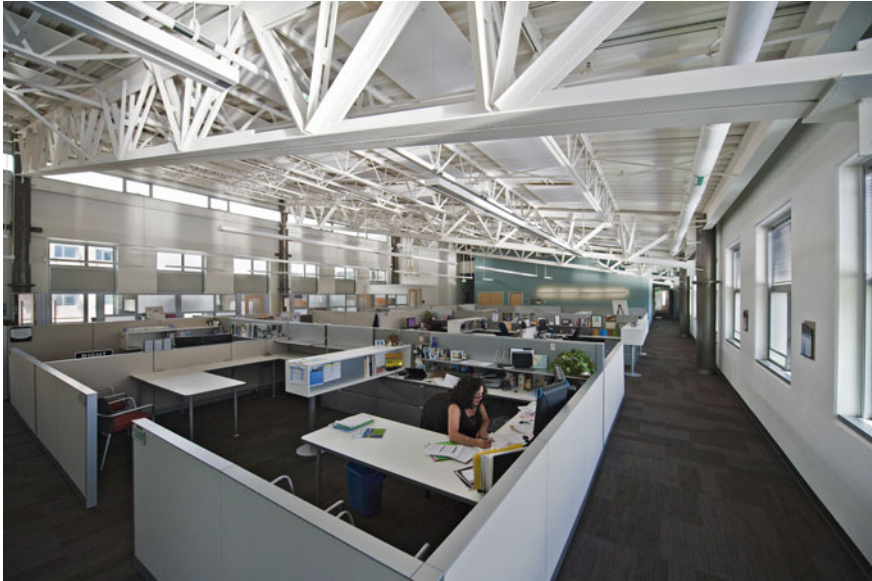
Fig. 5.19 Third floor interior. A narrow floor plate [18.3 m (60 ft)] and an open-office workstation layout enable the potential for daylighting and natural ventilation for all occupants. This image has been reprinted with permission from National Renewable Energy Laboratory
