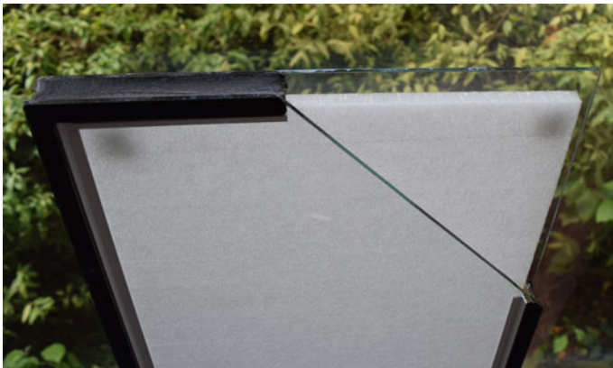
Fig. 3.20 Photograph of light-diffusing capillary slab integrated within standard double-glazing IGU (Okalux). The capillary slab can be incorporated into a range of standard IGU configurations (e.g. double and triple glazing, gas fill, with low-e coatings). Image credit Okalux
