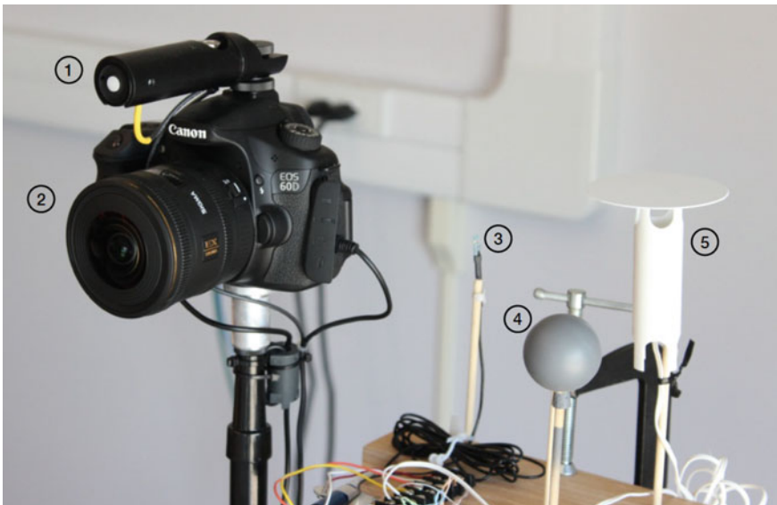
Fig. 4.35 Comfort sensing equipment installed in FLEXLAB: 1 Licor illuminance sensor for calibrating HDR images taken by 2 DSLR camera with 180° lens, 3 air velocity sensor, 4 mean radiant globe temperature sensor, and 5 shielded temperature sensor. Image credit LBNL
