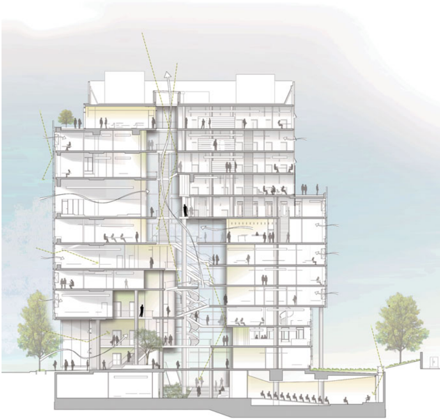
Fig. 5.4 Building section showing daylit atrium space that serves as the primary means of circulation and aids in the passive ventilation of interior spaces. Image credit Behnisch Architekten
