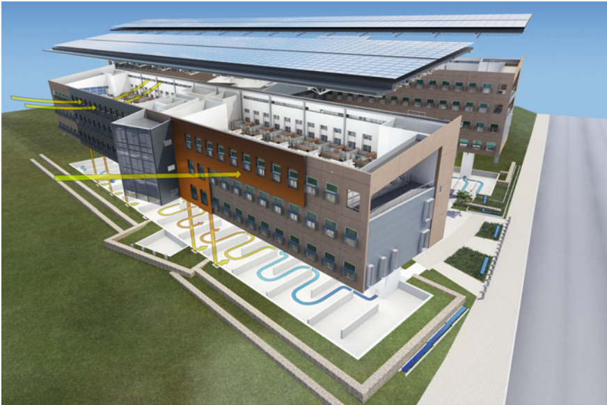
Fig. 5.24 Transpired solar collectors on south facade of building which supply passively-heated air to the thermal labyrinth below the NREL RSF building. Image credit RNL
