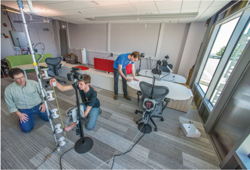
Fig. 4.34 Interior view of the U.S. Department of Energy's Facility for Low Energy Experiments in Buildings (FLEXLAB) showing Indoor Environmental Quality (IEQ) monitoring equipment including installation of shielded thermocouples at regular heights to assess thermal stratification. Image credit LBNL
