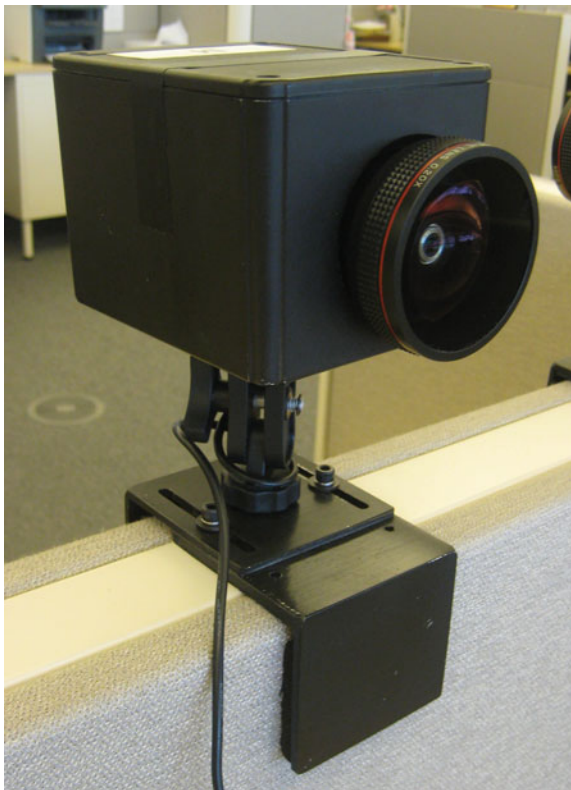
Fig. 2.28 Field installation of High Dynamic Range (HDR) enabled camera for acquisition of time-series measurements
