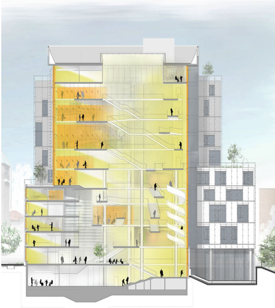
Fig. 5.3 Building section showing interior daylit atrium. Electrical lighting within 20 ft of facade glazing is controlled by photosensors to reduce output in response to available daylight. Image credit Behnisch Architekten
