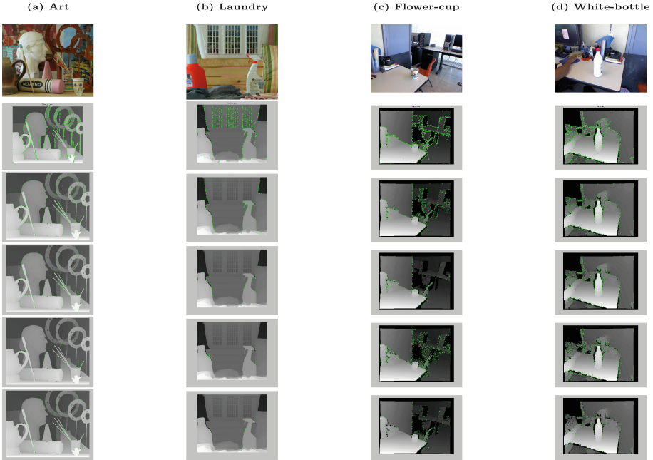
Fig. 4. Comparison between the proposal Sparse Keypoint Detector (SKD) and other techniques. First row color image. Second row SKD technique. Third row NARF detector. Fourth row Harris detector. Fifth row SURF detector and sixth row FAST detector.
