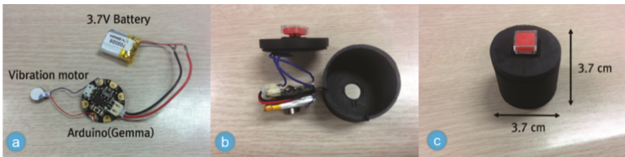
Fig. 2. Prototype (Vibration Token). (a) Circuit board and Actuator, (b-c) Case and Dimensions
