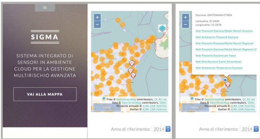
Fig. 3 On the left and center part of the image there is the homepage of the mobile version, that provides the first level visualization; on the right part there is the second level visualization, with the set of visualizations related to time series data, available for each station
