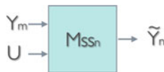
Fig. 1 A soft sensor capable to estimate a set of output parameters \tilde{Y}_n exploiting a set of parameters Y_m . U is a command signal
