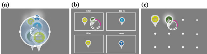
Fig. 4 Touchless SQUAD. a The user moves the pointer performing the selection phase, with the result that all the POIs which lie under the volume of the pointer are highlighted. b The user performs the disambiguation phase, which corresponds to the first refinement, and selects the area with the desired POI. c In a subsequent level of refinement, the user selects the target from the set of POIs in the grid
