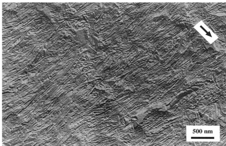
Fig. 3.4 Representative TEM morphology seen in quenched linear PE crystallized isothermally at 115°C. Sample had been sheared at 25 s -1 . The arrow indicates the shear flow direction in the melt. Y. An et al. (2006) Polymer 47: 5643–5656
