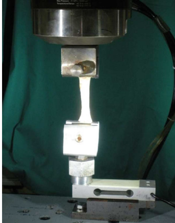
Fig. 9.6 Dog bone-shaped dermal automesh. Uniaxial pulling of the sample by mechanical testing device
