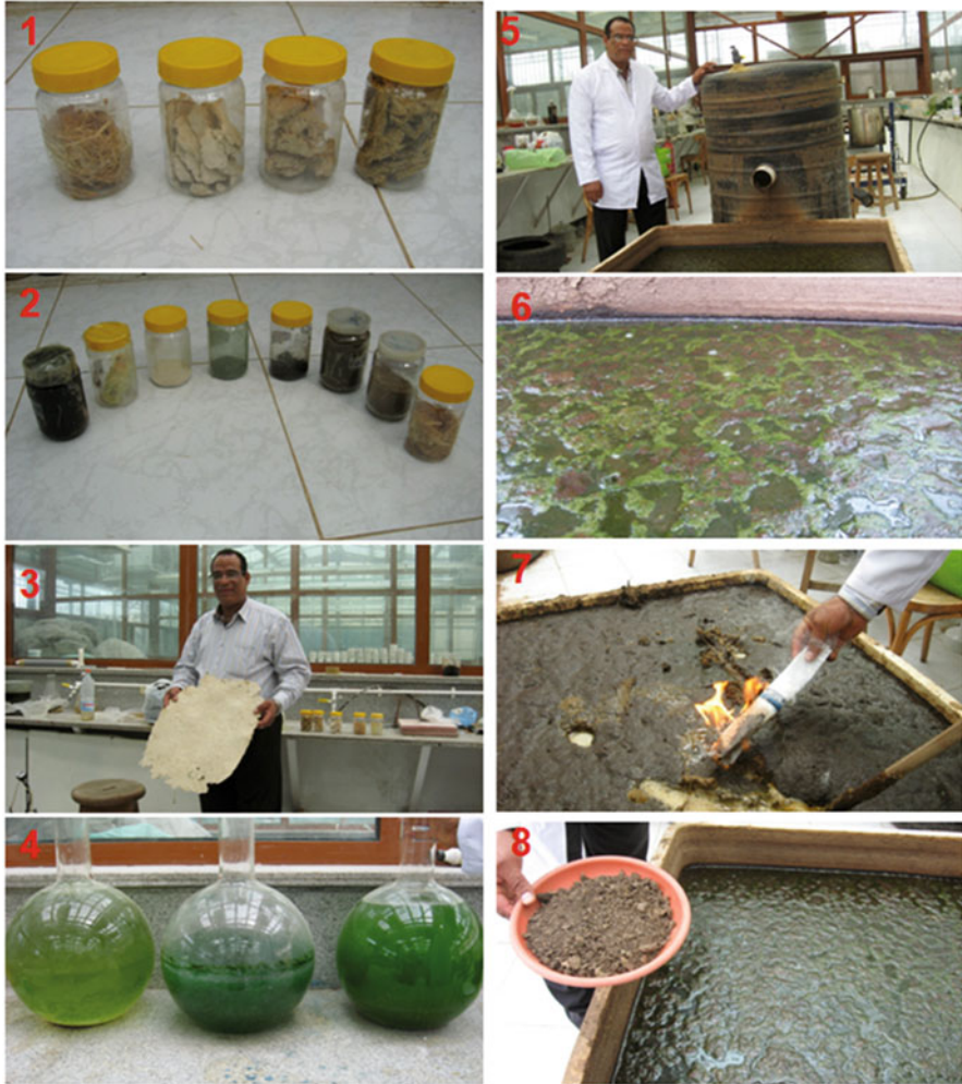
Fig. 10.2 A unique management for rice straw in Kafrelsheikh Uni. (photos from 1 to 3), where Prof. Belal and his co-workers have already extracted several products from this rice straw using special microbial strains. These products include cellulose A, B, and C (Photo 1), from left to right: humic acid, bioethanol, silica, lignin, compost, alternative soil and rice straw (Photo 2) cellulose (Photo 3), and algae (photo 4). Production a biogas from farm yard manure (Photos from 5 to 8), where biogas slurry enriched with algae can be obtained (Photos 5 and 6) and biogas can be noticed from the ignition in Photo 7 and dried biogas slurry (Photo 8) (Photos by El-Ramady)
