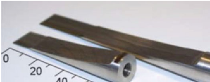
Fig. 3.49 20 kHz ( long ) and 35 kHz ( short ) ultrasonic cutting blades (reprinted from Cardoni et al. [92] with permission. © Elsevier)
