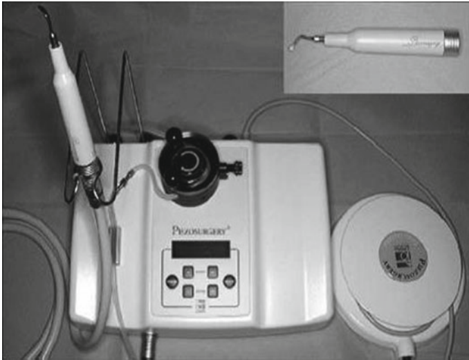
Fig. 3.50 The piezosurgery device with a piezoelectric hand piece (reprinted from Robiony et al. [96] with permission. © Elsevier)
