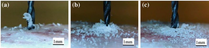
Fig. 4.23 Variation of chip morphology in bone drilling at various rotational speeds: a continuous-12 m/min; b fragmented-30 m/min; c powdery-48 m/min (reprinted from Liao and Axinte [46] with permission. © Elsevier)
