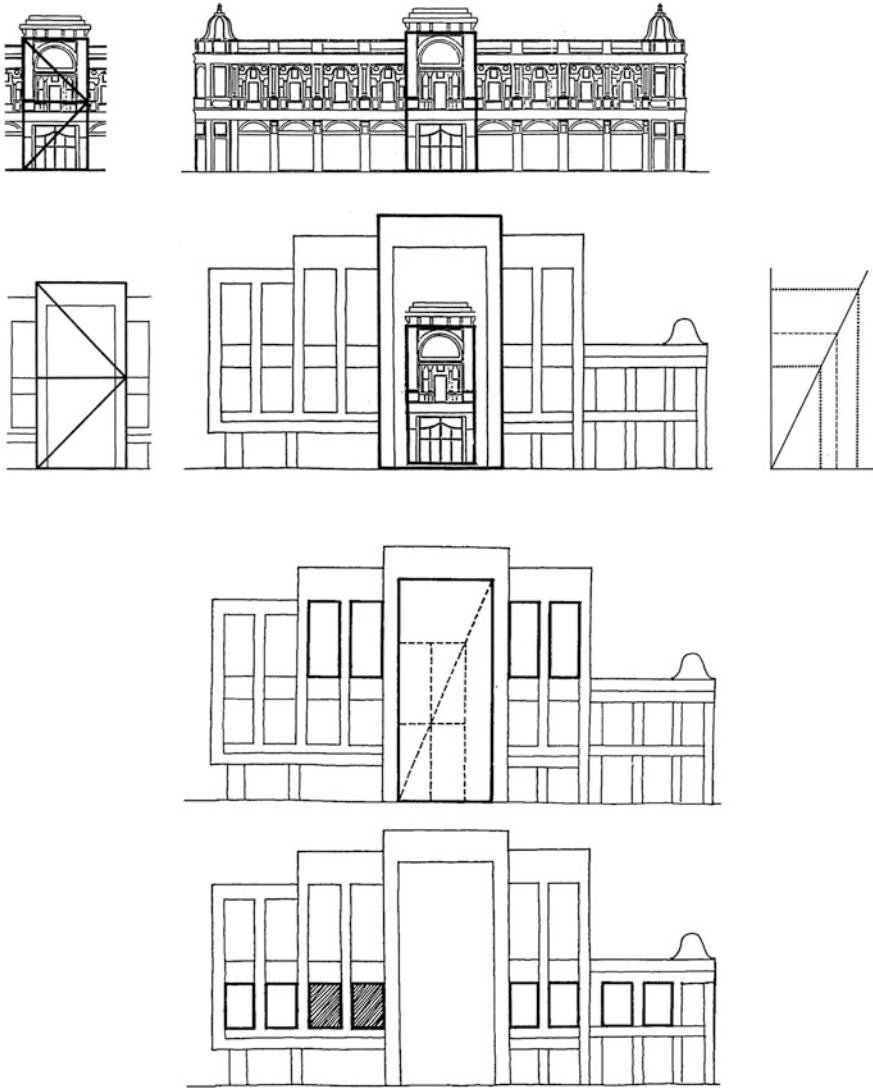
Fig. 9.23 Tehran. Hasan Abad Square. New shape based on the flow of the proportions from the old to the new
