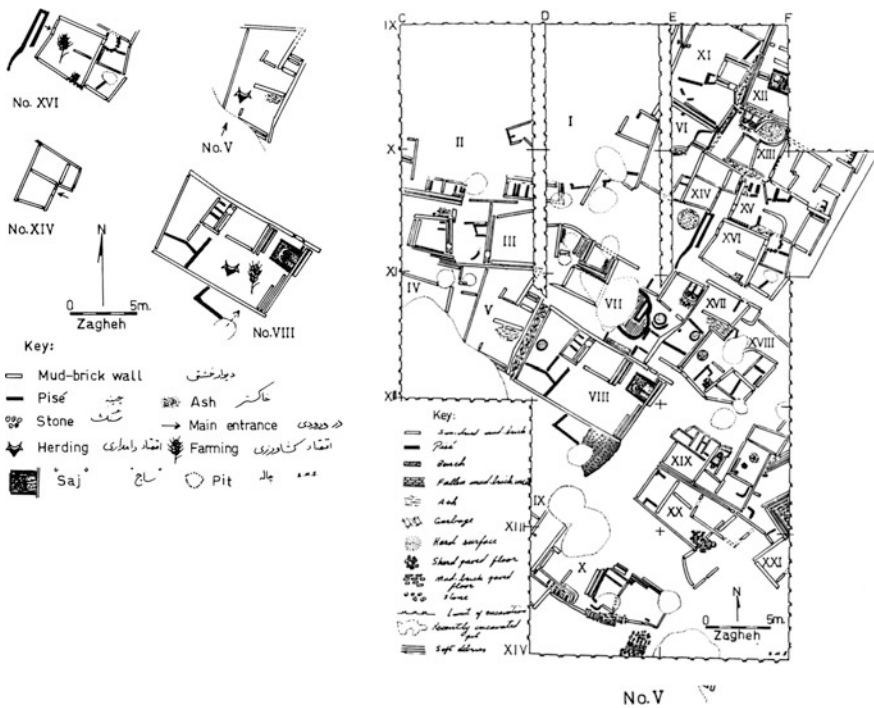
Fig. 1.3 Iran, Zageh Village. Detail plan of part of the housing area, the period around 5000 BC. The structure has been oriented favorably, considering sun radiation and unfavorable winds (Shahmirzadi 1986)
