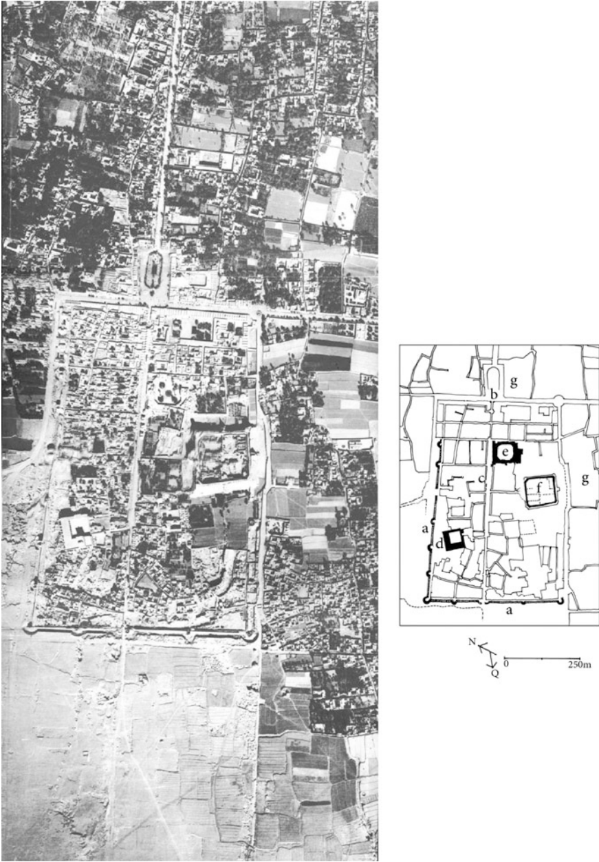
Fig. 4.20 Tabas. Spatial structure including: a Town wall (traces). b Main gate. c Bazaar lane. d Masjid-i Jamai. e Madrasah. f Citadel (Qal'ah). g Outer areas, gardens. (Aerial view from: National Cartographic Centre, Iran, 1973)
