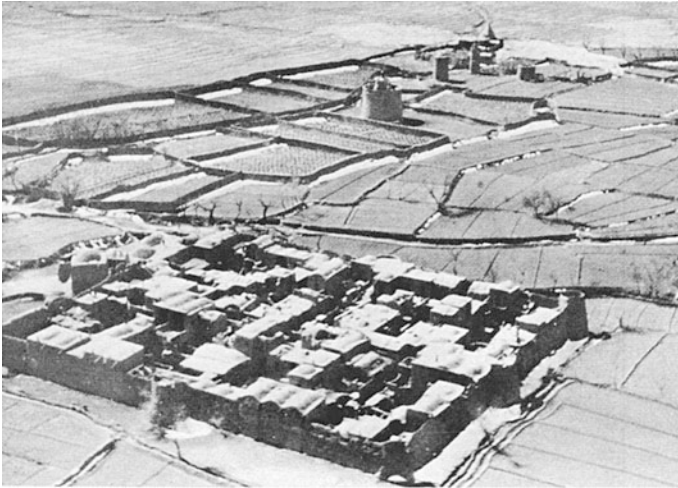
Fig. 3.3 Iran. “A long, close contact with nature evolved solutions such as those of the Iranian village in the Oasis of Veramin, where the village huddles together to leave the least surface to the scorching heat. The geometric minimum of the individual units is echoed in the total layout, bringing an appealing unity, and the closeness yields protection through mass. The thick walls tame and delay the thermal variations. The courtyards are shaded, providing cooling wells and establishing ‘introvert’ dwelling units looking inward from the hostile environment. This distinct order took form through the urgency of biological necessity” from Olgyay
