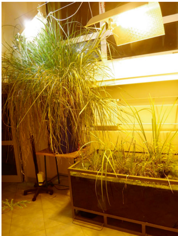
Fig. 15.1 Experimental mesocosm system: VF-CW (left) and FEM-CW (right), photo taken on day 342 of the experiment
